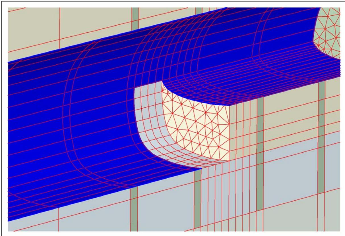
Figure 6: Simulation of the invert excavation
