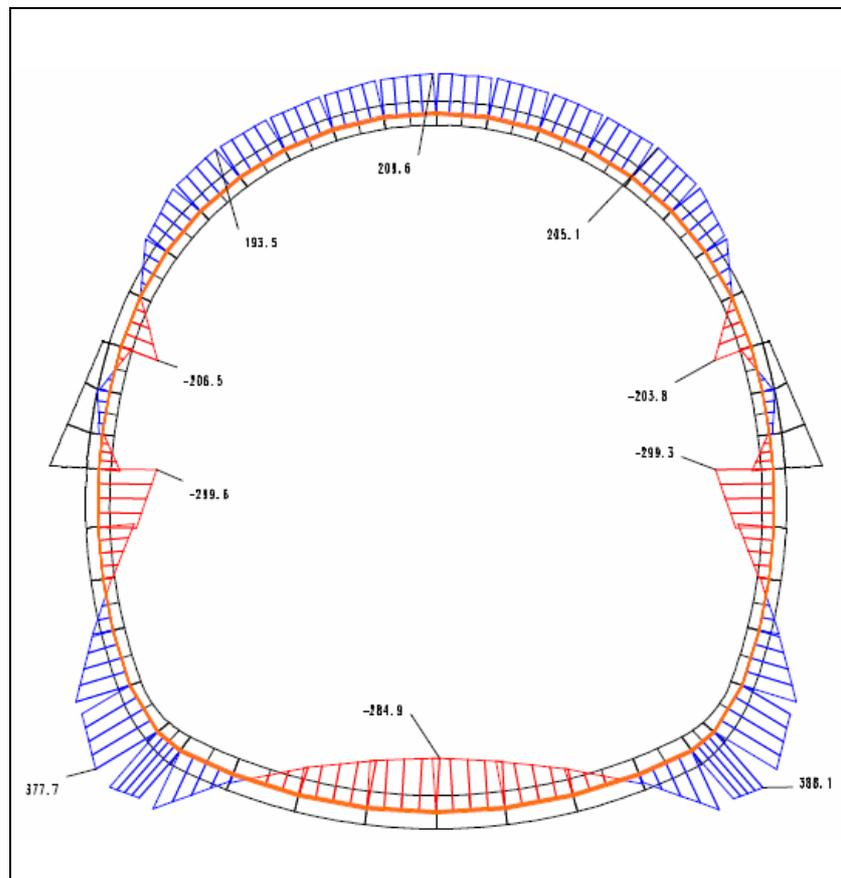
Figure 3: Final bending moments in completed primary lining
