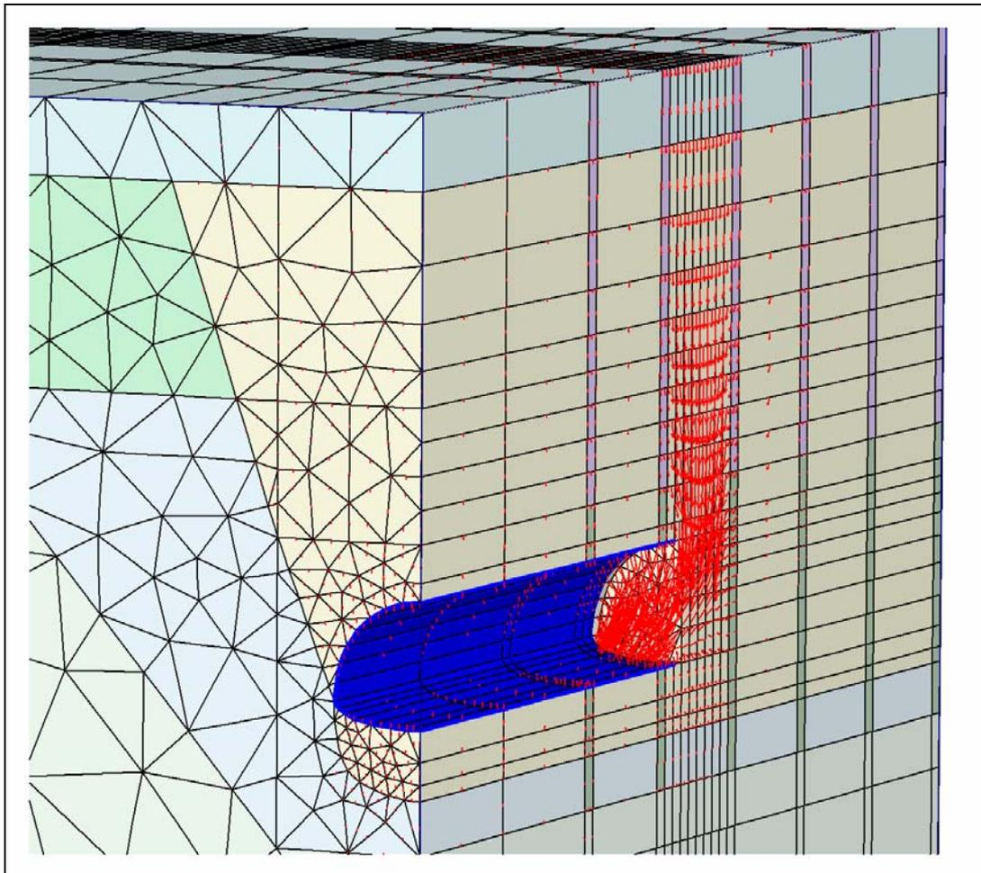
Figure 7: Propagation of the top heading face deformations
